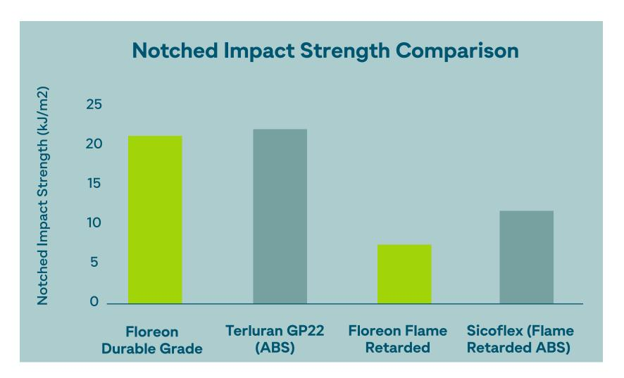
Floreon offer polylactic acid (PLA) based compounds with the performance of ABS. Our patented materials are suitable for both durable and disposable applications
